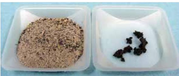
*Left shows a sample of the desiccant fines upstream of the dust filters. Right shows a sample of the solid contaminant that was captured using a boroscope while on-site at the facility.*
