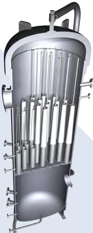
**Pentair Apex Zenith Element Filters in housing**
