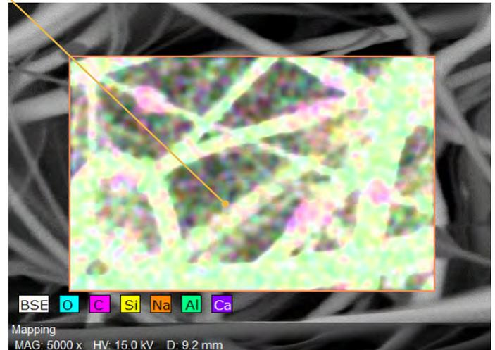
**EDS of media showing droplets to be carbon based**
